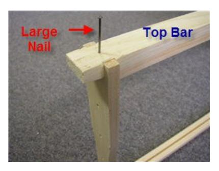
7. Now for each end, drive one more large nail through the side bar into the top bar (not the wedge which was removed, but the part that was NOT removed). This is an important nail, so don't skip it.
